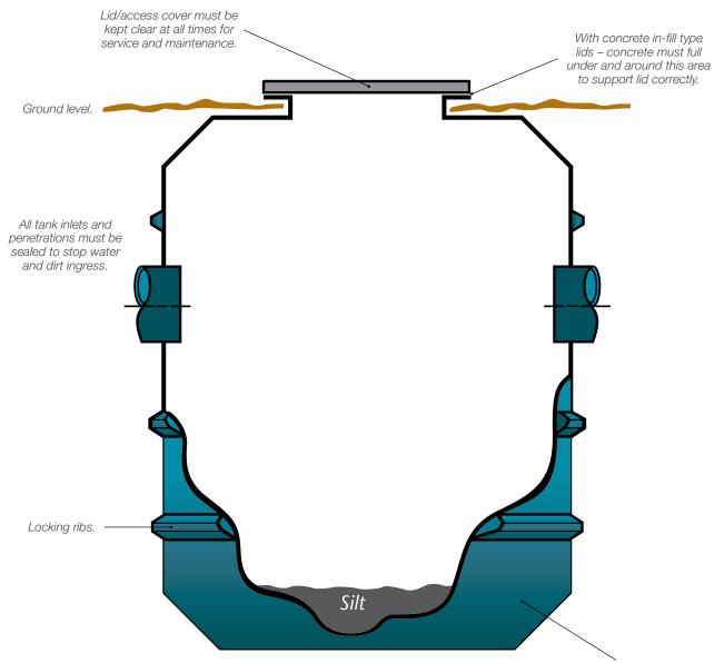
Minimum concrete grout level – fill tank with ballast weight (water) before concreting up sides of tank.
