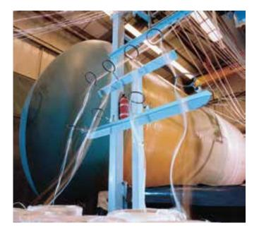
This process produces not only circumferential strength as found in helical wound tanks, but also longitudinal strength. The interlaminar shear strength permits tanks to be cut for manholes and pipework without any undue loss in strength.
