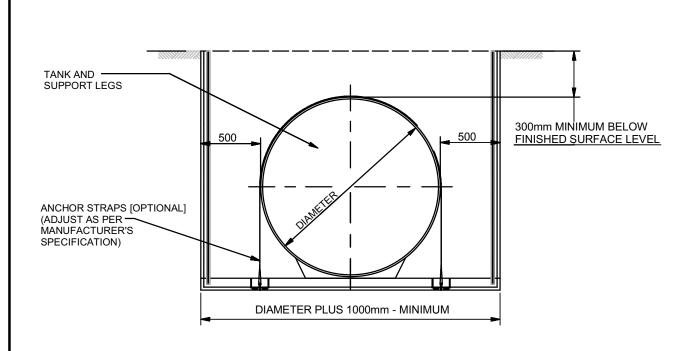
D: FIT TANK INTO EXCAVATION AND FIX INTO POSITION WITH ANCHOR STRAPS
